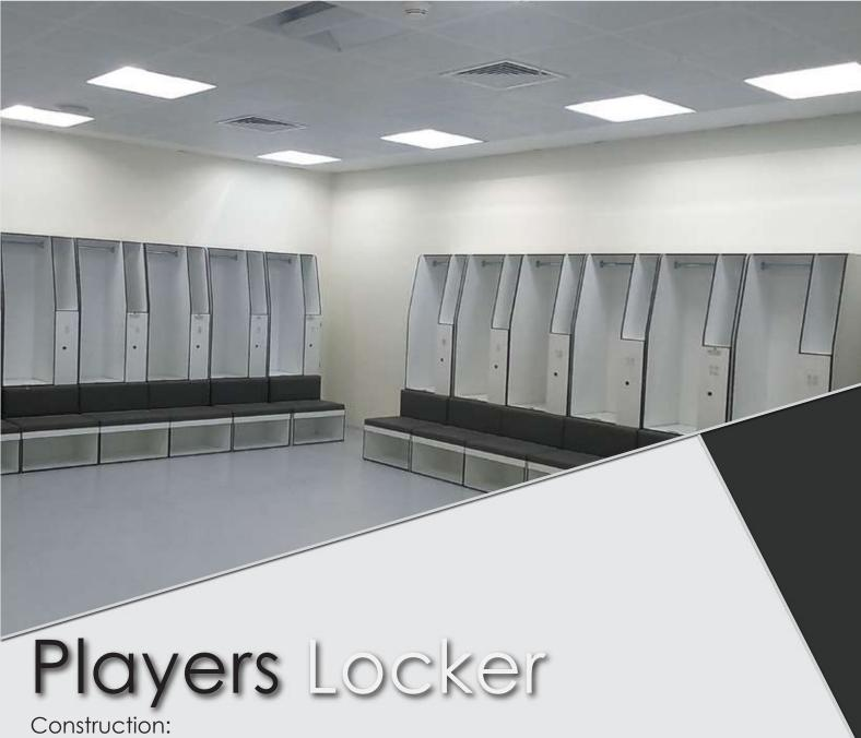
Player's locker is made of 13mm thick High Pressure Laminate with back panel made of 6mm thick HPL composed of layers of kraft paper impregnated with phenolic resin, having superior resistance against impact, every day wear and tear, scratches, stains and water, and maintaining its integrity even in the most heavy-duty application.
